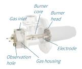
posed of a gas pipe and a burner head, which is used for mixing the gas and air and stabilizing the flame. Electrodes are installed on the burner insert, and double-electrode flame ignition/detection is adopted generally.
