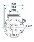
Pilot burner gas connection Rp1/4", air connection Rp1/2".
