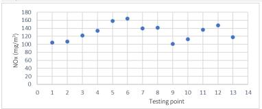
Measured data of stainless-steel continuous annealing production line.
